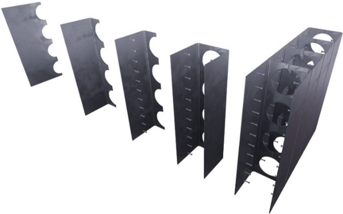
Figure 2-5: Construction of Steel Bricks™ (Reference 5-1)
