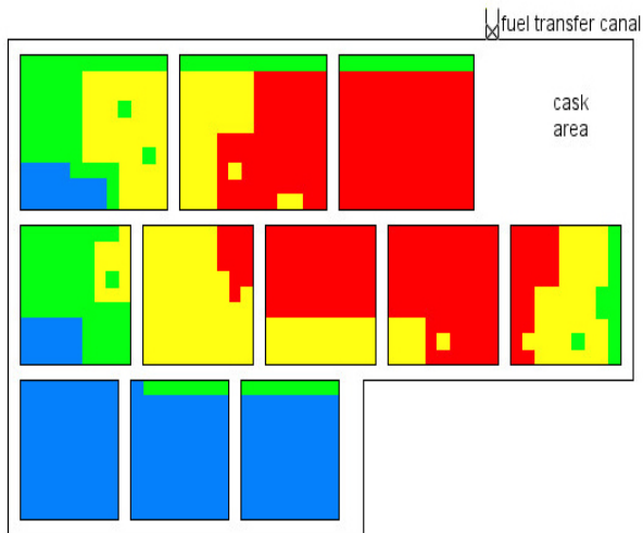
Figure 4–7. Example of a RACKLIFE simulated spent fuel pool showing regions of high (red), medium (yellow), low (green), and near-zero (blue) loss.
