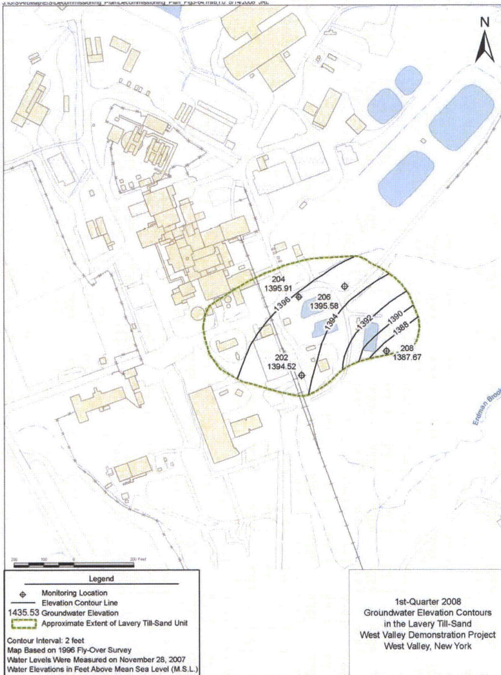
Figure 5C9-2 – Current Inferred Areal Extent of the Lavery Till Sand in the North Plateau
