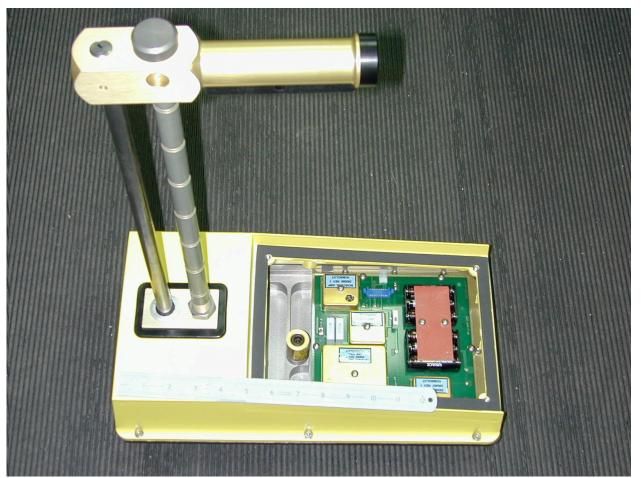
Shown above is the type of moisture density gauge involved, with its lid removed. One of the sources would be at the bottom of the long handle at far left, while the other source would look like the small cylindrical component found in the center of the device.
