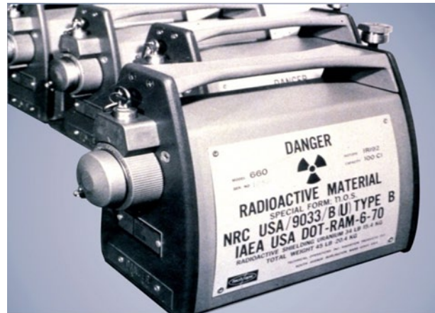
Radiography cameras spot cracks in metal or pipe
