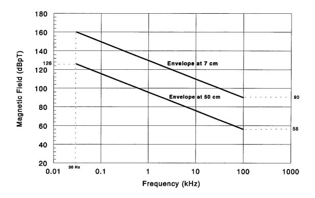
Figure 4.6 RE101 Magnetic Field Emissions Envelopes
