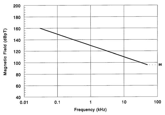
Figure 4.13 RE01 Magnetic Field Emissions Envelope
