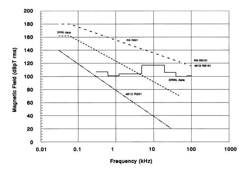
Figure A.3 Comparison of low-frequency radiated susceptibility envelopes
