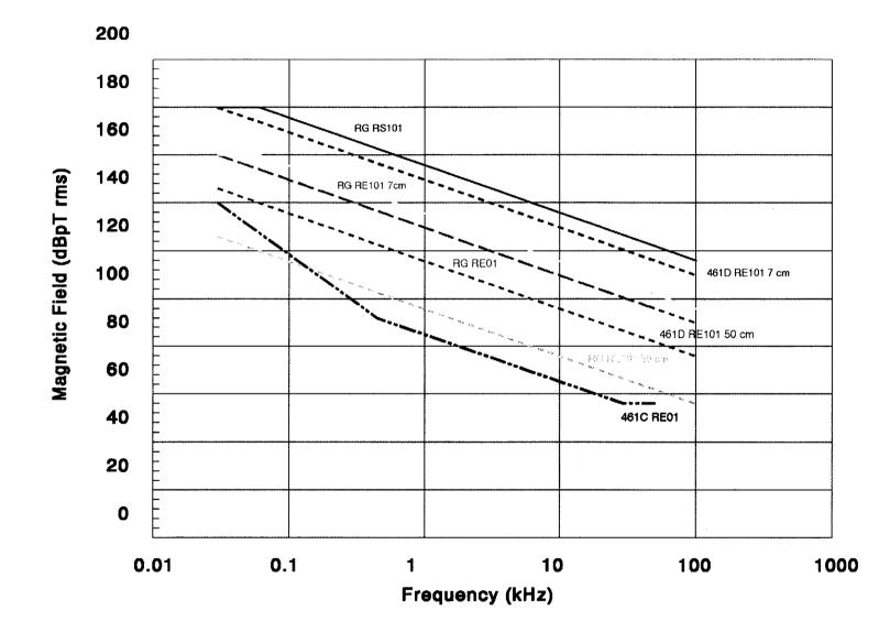
Figure A.7 Comparison of low-frequency radiated emissions envelopes
