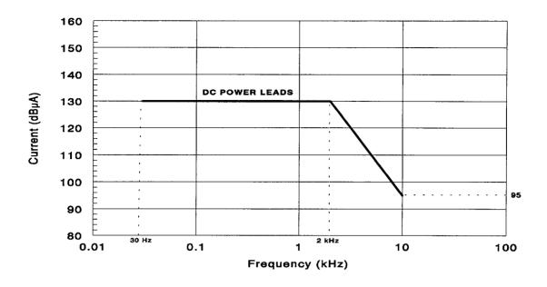
Figure 4.1 CE101 Emissions Envelopes for dc Power Leads
