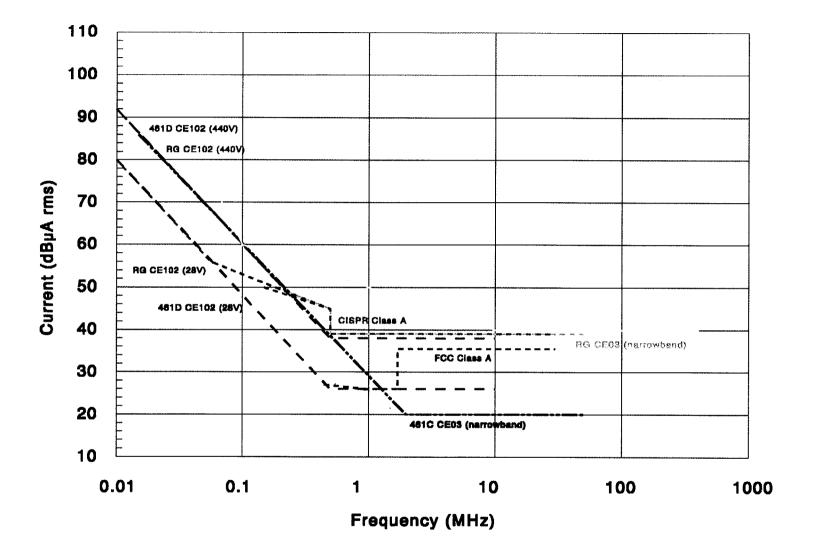
Figure A.6 Comparison of high-frequency conducted emissions envelopes
