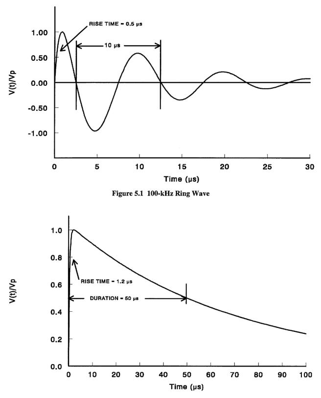
Figure 5.2 Combination Wave, Open-circuit Voltage
