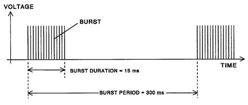
Figure 5.5 Pattern of EFT Bursts
