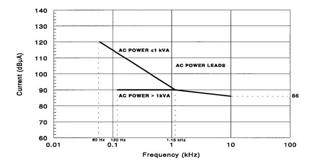
Figure 4.10 CE01 Emissions Envelope for ac Power Leads
