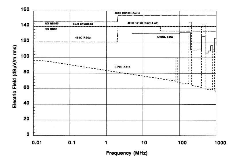
Figure A.4 Comparison of high-frequency radiated susceptibility envelopes
