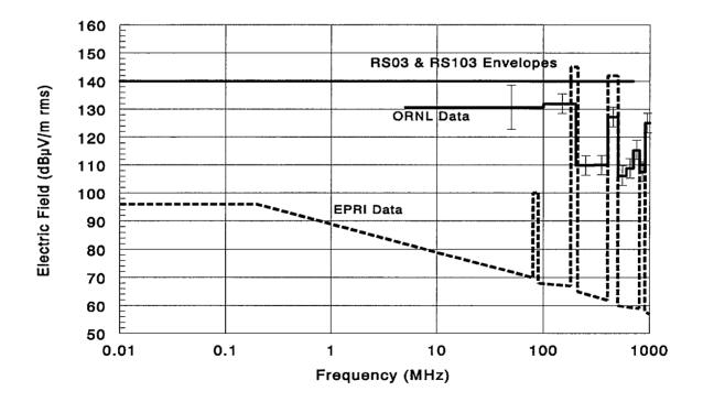
Figure 6.1 Data vs Envelopes, Radiated Electric Fields
