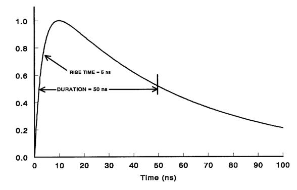
Figure 5.4 Waveform of the EFT Pulse
