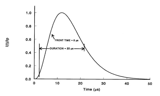
Figure 5.3 Combination Wave, Short-circuit Current
